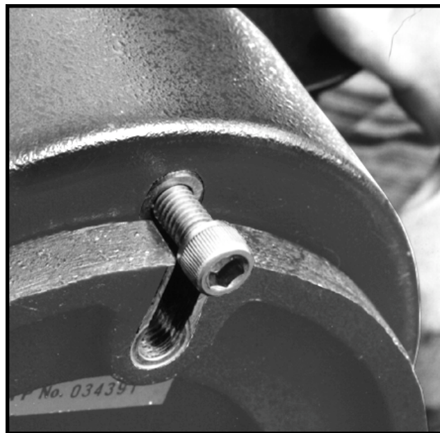
Figure 6 The wedge with the bolt installed on the telescope base being slid into the slot on its face.
