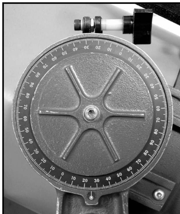
Figure 4 A photograph of the declination setting circle. The use of this setting circle is detailed in the section on setting circles.
